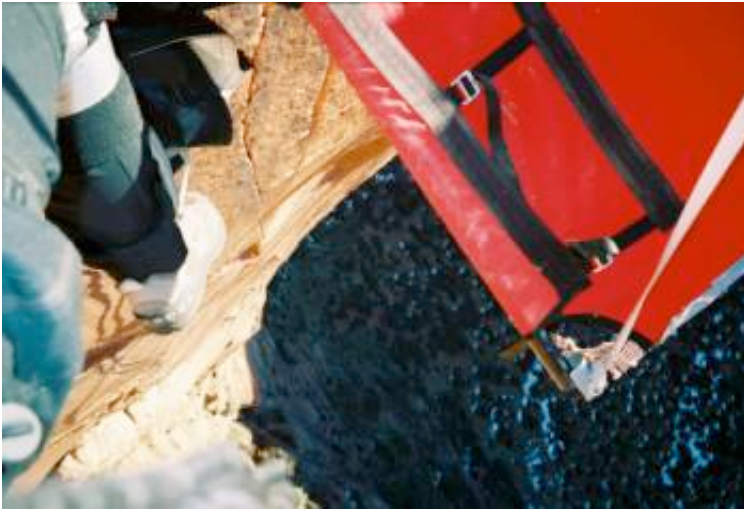
Metolius end tubes demonstrating corner instability despite tight bed tensioners. (Lunar Ecstasy Solo, Zion NP, Jan 2004)
