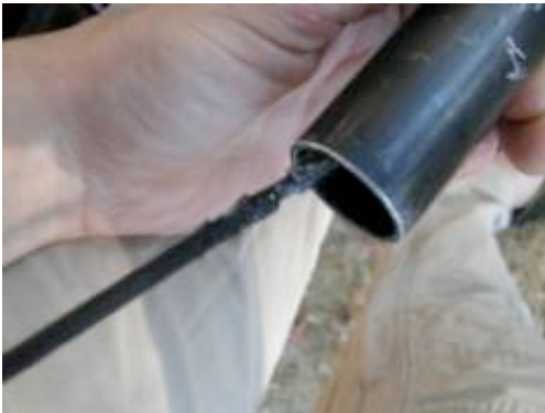
Photo of Metolius Bombshelter shock-cord wear. You can see the residue from where I tried to reinforce the cord with duct tape.
